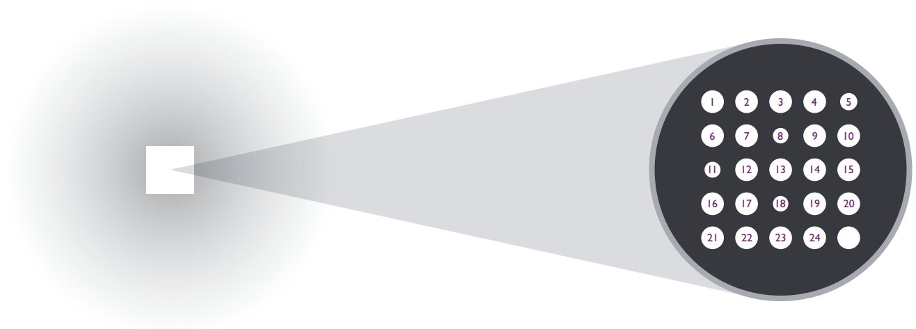
Discrete Test Regions (DTR) on each Biochip for individual analytes
